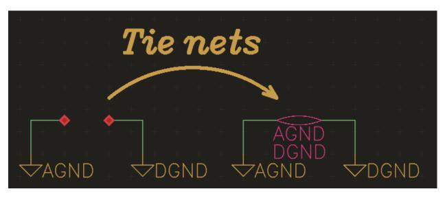
The net that's listed first (AGND in this case) is the primary net of a net tie. See *Board Net ties* for what that means and how to represent net ties on the board. The "flip net tie" tool swaps primary and secondary net of a net tie.
