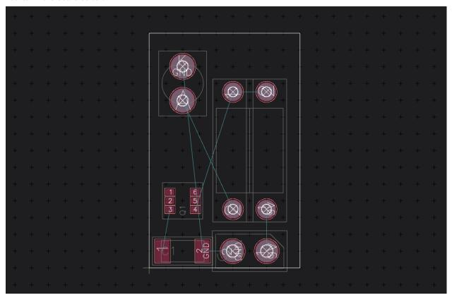
If you want to place a part on the bottom of the board, press e to flip it to the bottom side. If you are working a lot on the bottom you can use the "View bottom" tool to flip the whole board around.
