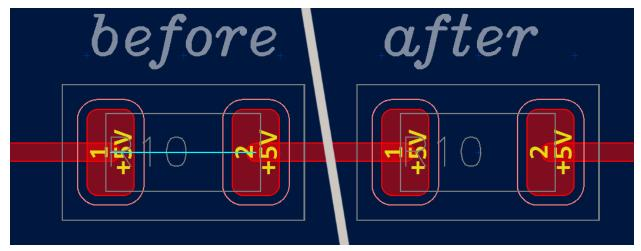
Create a "Shorted pads" rule to specify that the pads of a part are electrically connected.
