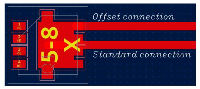
Keep in mind that tools based on the KiCad router such as "Route track" or "Drag track" aren't aware of this and will break the pad-track connection.
