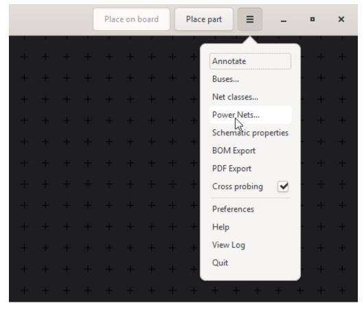
In the window that pops up press the "Add power net" button, give the net a name and select a symbol style. Place power nets with the "Place power symbol" Tool (type p o).
