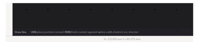
The Action bar will show additional keys you can press to change the behaviour of the tool. In this case you could press w to change the width of the stroke or / to restrict the movment of the manipulator to one direction.
