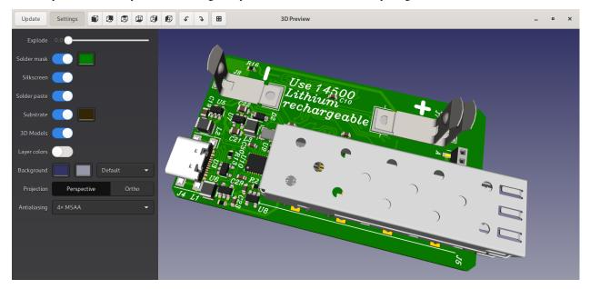
When the design is done, export the board and all models as STEP file for use in mechanical CAD:
