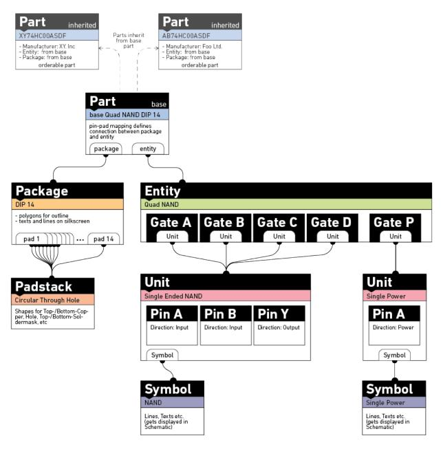
For example you can define one "Quad NAND" Entity and reuse it for each new NAND Part, without having to redefine the Gates time and time again. The Quad NAND Entity in turn is composed of multiple Single Opamp NAND Units and one Power Unit. If you now want to make a Dual NAND Entity, you can just reuse the already existing Units and this guarantees you consistency with the other NAND parts in your pool.
