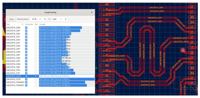
Interactively measure and tune individual tracks, differential pairs or buses:
