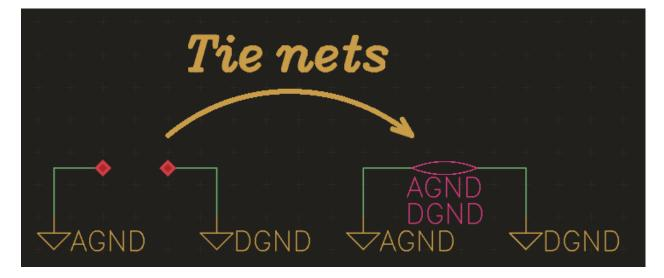
The net that's listed first (AGND in this case) is the primary net of a net tie. See *Board Net ties* for what that means and how to represent net ties on the board. The "flip net tie" tool swaps primary and secondary net of a net tie.
